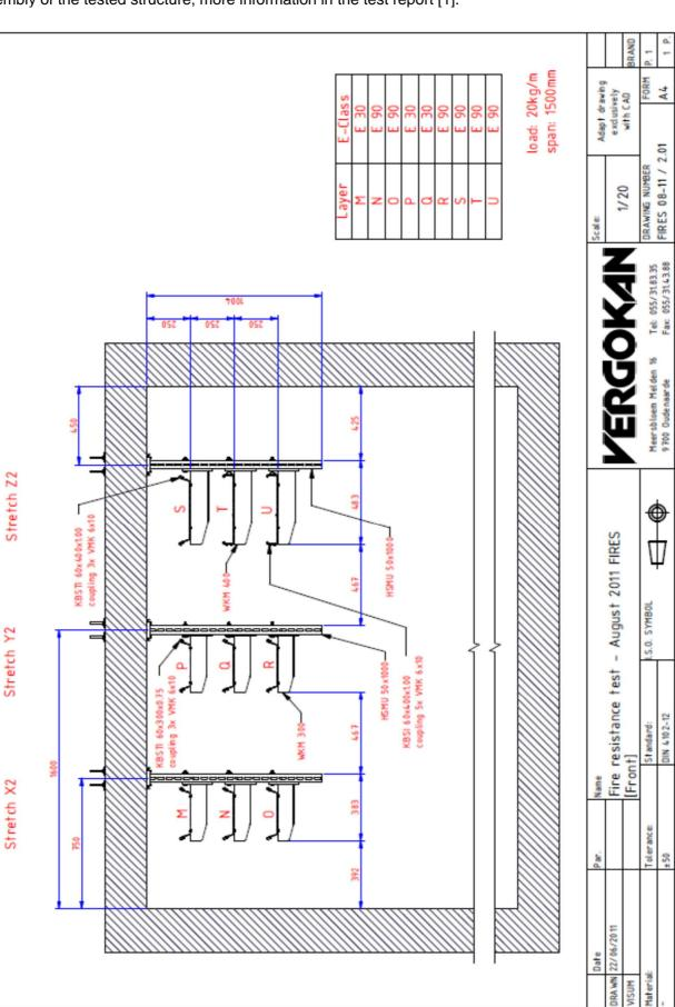
Assembly of the tested structure, more information in the test report [1].
