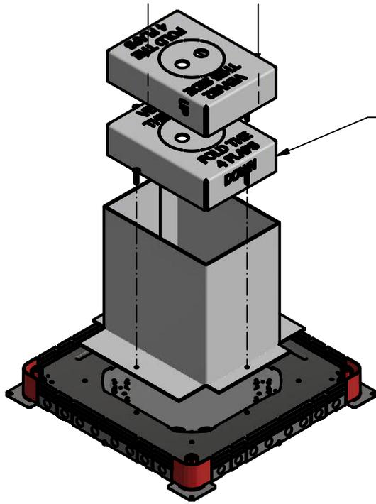
Press the stiffening element down on to the NEO top plate
