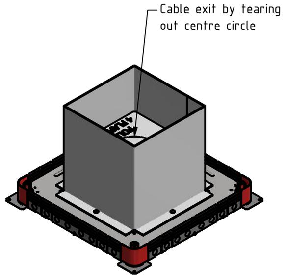
Cable exit by tearing out centre circle
