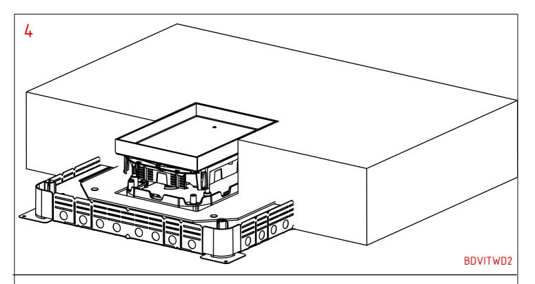
1. Installing the supporting frame
