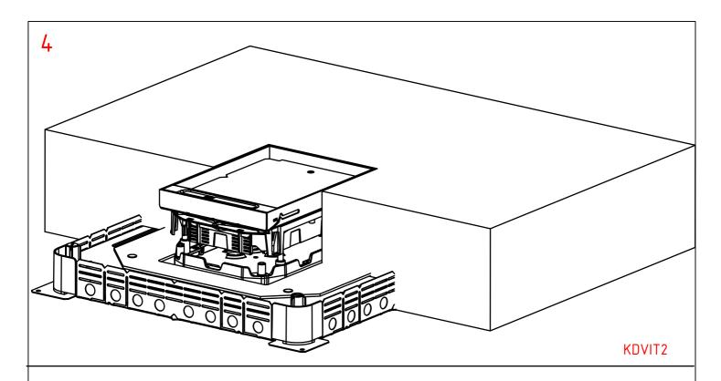
1. Installing the supporting frame
