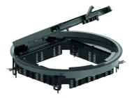
Build-in frame + hinged cover + cable outlet unitColor: Grey RAL 7011/ Black RAL 9011Max. load: 1500 N (small surface area)Max. load: 2000 N (large surface area)Active condition: IP 20Non-active condition: IP 30Depth of floor covering: Min. 5 mm - Max. 12 mmThickness steel plate : 3 mmStandard finishPolypropylene
