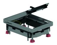
Build-in frame + tileframe + cable outlet + alu frame Max. load: 2000 N (small surface area) Max. load: 3000 N (large surface area) Active condition: IP 20 Non-active condition: IP 30 Depth of floor covering: Max. 26 mm
