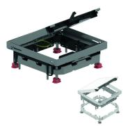
Build-in frame + tileframe + cable outlet + alu frame Max. load: 2000 N (small surface area) Max. load: 3000 N (large surface area) Active condition: IP 20 Non-active condition: IP 30 Depth of floor covering: Flat
