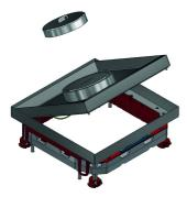
Build-in frame + tileframe + water resistant cable outlet + alu frame + tube cover key Max. load: 2000 N (small surface area) Max. load: 3000 N (large surface area) Active condition: IP 23 Non-active condition: IP 53 Depth of floor covering: Max. 26 mm
