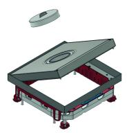
Build-in frame + tileframe + water resistant cable outlet + alu frame + tube cover key Max. load: 2000 N (small surface area) Max. load: 3000 N (large surface area) Active condition: IP 23 Non-active condition: IP 53 Depth of floor covering: Flat
