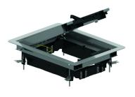
Build-in frame with border + tileframe + cable outlet Max. load: 2000 N (small surface area) Max. load: 3000 N (large surface area) Active condition: IP 20 Non-active condition: IP 30 Depth of floor covering: Max. 26 mm
