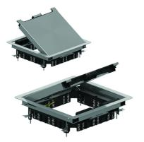
Build-in frame with border + tileframe + cable outlet Max. load: 2000 N (small surface area) Max. load: 3000 N (large surface area) Active condition: IP 20 Non-active condition: IP 30 Depth of floor covering: flat
