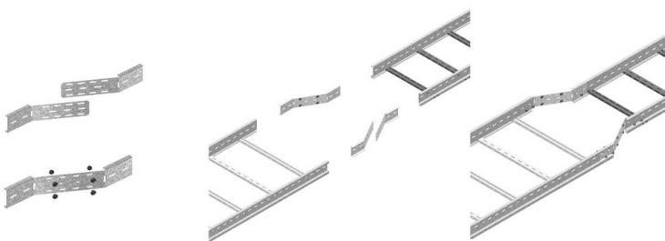
**A fixer avec:**
