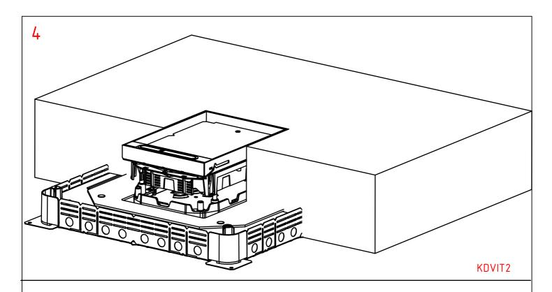
1. Installing the supporting frame
